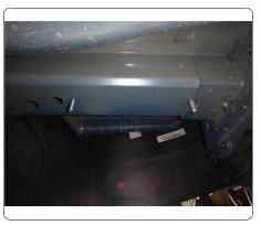
2. Raise hitch into position and secure with (4) 7/16" flange nuts, (2) each side.Torque 7/16" hardware to 70 ft-lbs.
