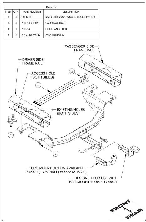
Fishwire (2) CM-SP2 spacers and (2) 7/16" carriage bolts on each frame rail through access holes and out mounting holes. (SEE FISHWIRE TECHNIQUE DIAGRAM)
