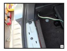
5. Adhere the black converter box to the frame of the car using the double-sided tape provided. Secure any loose parts of the T-connector with the cable ties provided.
