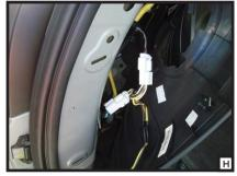
2. Separate the vehicle's connectors taking care not to damage the alignment tabs. Starting on the driver's side insert the T-Connector end with the yellow wire between the separated connectors. Make sure the connectors are fully inserted with locking tabs in place (H).
