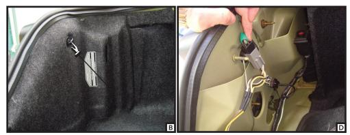
1. Open the trunk and remove the vehicles rear scuff panel. A On both sides of the trunk remove plastic wing nuts holding the felt trunk liner in place. BPull back on the trunk liner and locate the vehicles taillight wiring harness. The harness will have connectors that are similar to those on the T-connector.
