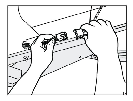
1. Locate the vehicle's tail light wiring harness along the inside of the left rear frame rail. (T3) This harness will have a connection point with connectors matching the ends of the <u>T-connector adapter</u>.
