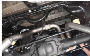
CROSS MEMBER Figure 3.2: View under bed towards axle.
