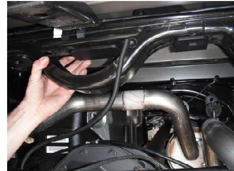
Figure 8.1: Axle Vent Hose Relocation
