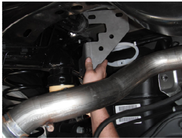
Figure 6.4: Driver side plate as viewed from floor up toward driver side frame. (Fuel tank is not shown.)
