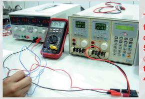
The highest temperature during 5 minutes @ 24V testing: 47 C
