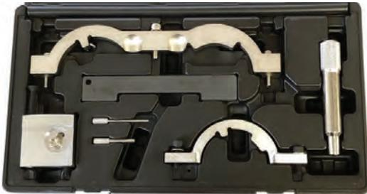
**5054 GM CAM PHASER LOCKING TOOL - 2.0L & 2.4L ECOTEC**
