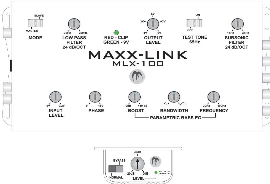
The Maxx-Link allows you to Link or Strap two matching mono amps that do not already have the “Master / Slave” feature built in.
