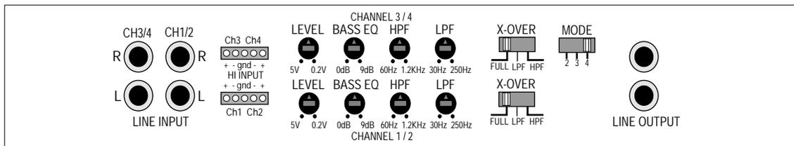
The 4 channel amps have the same features as the 2 channel models except that there are 2 sets of controls. 1 set for channels 1 & 2 and 1 set for channels 3 & 4.
