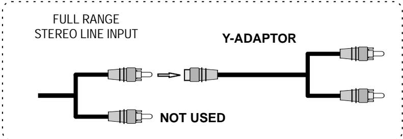
Note: You can use the Radio/CD designated mono line output or a full range stereo line output. For full range stereo line output, you will need an optional "Y-Adaptor" as shown.
