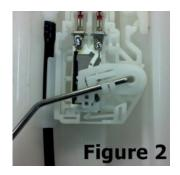
This fuel module ships with the arm detached from the module. To assemble float arm onto the fuel module insert the float arm into the hole (see Figure 1) and rotate the arm down so it engages the 2 clips on the bracket (see Figure 2). Ensure that it has a full range of motion and the float arm does not contact the body of the fuel module.
