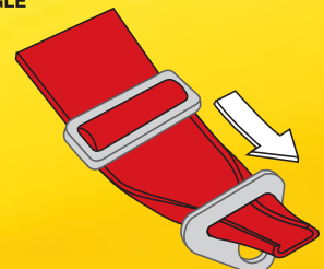
STEP 2: Pull strap to 8"-10" beyond buckle, fold edges and insert into mounting bracket.
