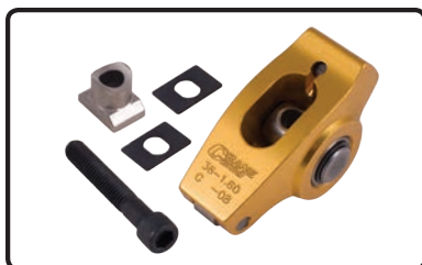
Extruded Gold Race rocker for Ford 289-302-351W-5.0L H.O., non-adjustable, 1.7 ratio. Uses stock-type 5/16" bolt. For hydraulic and hyd. roller cams only.
