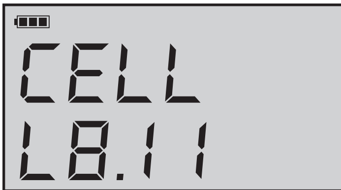
Figure - 3: Shows the display and control unit battery voltage.
