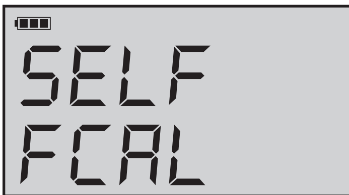
Figure - 9: Notifies the user that a full scale calibration is being performed.
