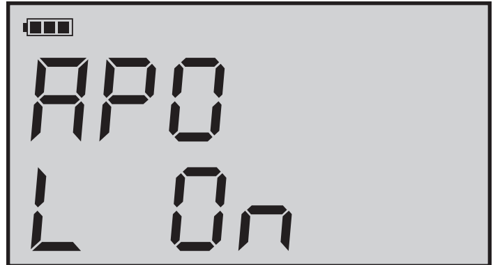
Figure - 2: Automatic Power Off enabled. Press [TARE] key to change. (See page 8 for details)
