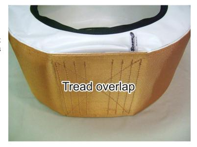
**Solution:** Air Channel placement can compensate for the Tread overlap heavy spot. At installation, simple arrange the Air Channel to be 180° across from the Tread overlap.
