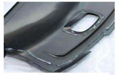
Apply the silicone provided in your kit to the underside of the dash cover only around the edges and vent holes. Do not apply silicone to the middle areas of the dash cover. The supplied tube of silicone is enough to install the dash cover.
