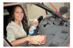
Clean your existing dash and the underside of your new Coverlay dash cover with an ammonia-based cleaner such as Windex®.
