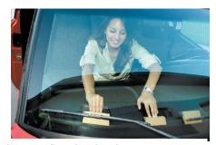
Insert cardboard wedges between your Coverlay dash cover and your windshield to create pressure on the dash cover edge against the window.
