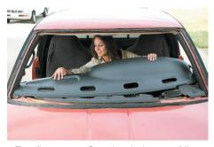
Test fit your new Coverlay dash cover. Minor adjustments sometimes are needed; use a utility knife or sandpaper. The dash cover should fit snugly over the entire dash. Practice putting it in place before moving to the next step.
