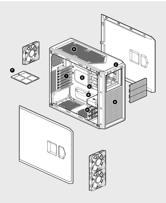
> Remove the thumbscrews and slide the side panel forward toward the front of the case to remove.
