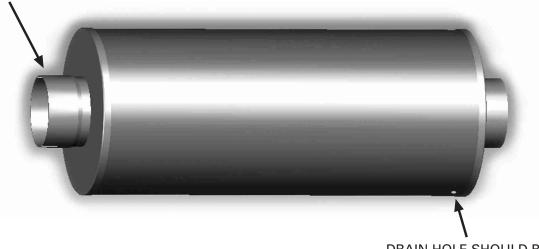
DRAIN HOLE SHOULD BE POSITIONED AT BOTTOM REAR OF MUFFLER ONCE MOUNTED.
