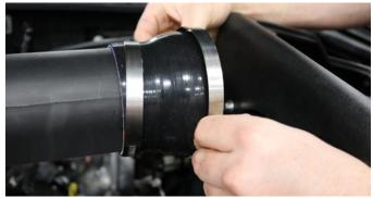
10. Locate CORSA air duct, silicone reducer, remaining #56 clamp, and #64 clamp. Place smaller end of reducer approximately one inch onto air duct along with the # 56 clamp. Loosely place #64 onto larger end of reducer.
