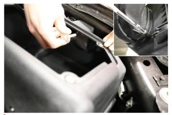
Locate the bolt from removal step 7 and attach the CORSA air box to the inner fender using a ratchet and 13mm socket.
