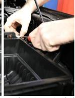
**6.** Disconnect wiring harness from lower half of factory air box by using a trim removal tool on the wire clips.
