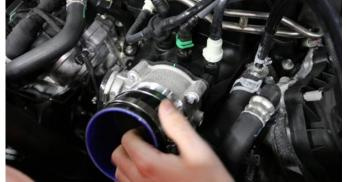
**9.** Locate the Ø3.5" straight sleeve and two #56 clamps. Install straight sleeve with one clamp onto throttle body and tighten clamp with flathead screwdriver or ratchet and 8mm socket. Loosely place other clamp onto straight sleeve.
