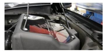
**13.** Locate the CORSA lid assembly, lid screws, and rubber washers. Install lid assembly onto air box using a Philips head screwdriver.
