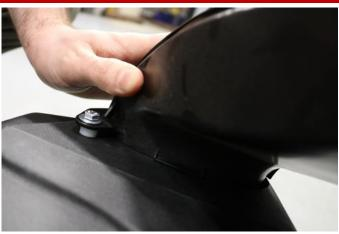
2. Locate the factory scoop from removal step 10, the 6mm x 25mm bolt, one .25" x .63" flat washer, the .25" x .75" flat washer, one .25" lock washer, the .25" spacer, and the 6mm nut. Attach air scoop to air box placing the spacer between the scoop tab and air box. Tighten hardware with 10mm wrenches.
