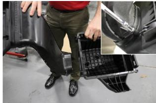
**10.** Remove bolt securing scoop to air box using a ratchet and 8mm socket. Separate scoop from air box.
