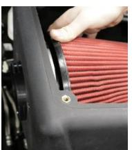
1. Insert the filter into the air box with the adapter side down. Rotate the top of the filter down into the air box and rotate the filter around and push the adapter through air box.
