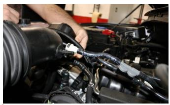
Disconnect both vent connections from rear of factory air duct.
