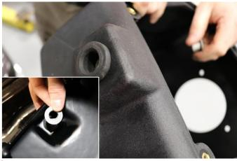
Locate CORSA air box and rubber grommet and metal bushing from removal step 9. Install grommet into air box the bushing into grommet from inside box.
