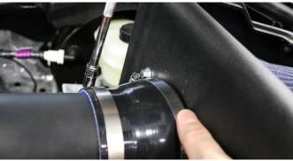
11. Install air duct into vehicle by placing the reducer onto the filter adapter and the opposite end into the straight sleeve clamped to the throttle body. Adjust duct as necessary and tighten all clamps using a flathead screwdriver or ratchet and 8mm socket.
