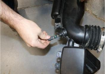
Remove the air temperature sensor from the factory air duct. Pay attention to the orientation of the sensor prior to removal to aid in installation.
