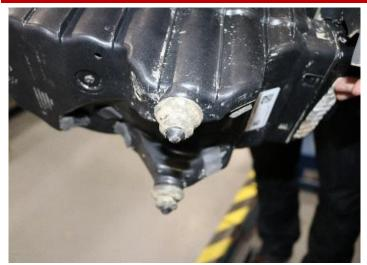
Remove the two mounting grommets from the bottom of the factory air box.
