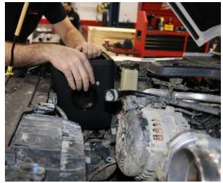
Locate the CORSA air box and install into vehicle by fitting the posts on the bottom of air box into the factory grommets installed in step 1.
