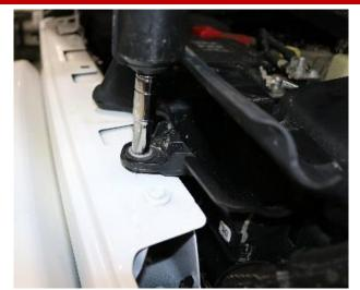
Remove the bolt securing the factory air box to the inner fender with a ratchet and 10mm socket.
