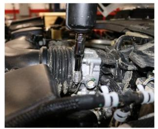
Loosen clamp securing factory duct to throttle body using a flathead screwdriver or ratchet and 8mm socket.
