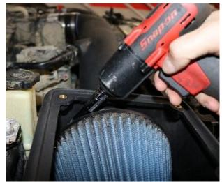
**14.** Ensure filter is fully seated onto adapter and tighten clamp using a flathead screwdriver or a ratchet and 8mm socket.
