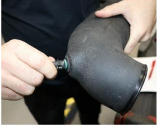
2. Locate the air temperature sensor from removal step 10 and CORSA air duct and install the sensor into the air duct
