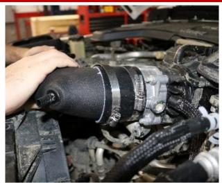
Install the straight sleeve onto the throttle body. **9**.
