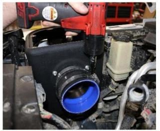
6. Locate the Ø3.5" Hump Hose and two of the #56 clamps. Install the hump hose and one #56 clamp onto to filter adapter. Snug the clamp to hold the hump hose in place, but do not fully tighten. Place the other clamp onto hump hose.
