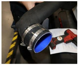
Locate the CORSA air duct, Ø3.25" straight sleeve, and two remaining #56 clamps. Install straight sleeve and one #56 clamp onto air duct and snug clamp to hold straight sleeve in place. Place the other clamp onto straight sleeve.
