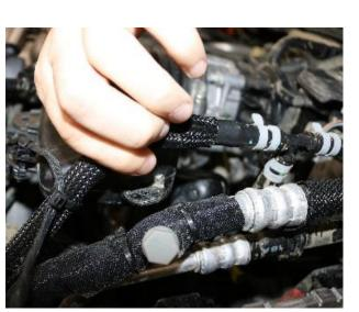
**3.** Using a trim removal tool, remove the clip securing the coolant hose to the factory air duct.
