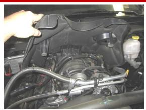
**5.** Remove the engine cover by pulling up the forward.
