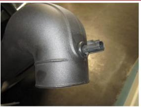
9. Locate the ATS sensor from removal step 1 and the CORSA air duct and install the sensor into the ½" grommet on the air duct paying attention to the direction of the sensor.
