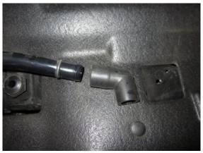
**6.** Remove the breather hose from the driver's side vent and remove the elbow from the breather hose.
