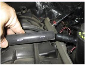
2. Locate the supplied 3/4" x 21" breather hose and install onto straight fitting. Install factory breather elbow back onto driver's side vent.
