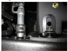
7. Locate the shorter L-bracket, the remaining factory air box tray mounting bolt from removal step 7, 6mmx25mm bolt, flat washer, lock washer, and 6mm nut. Attach the L-bracket the factory tray with the factory bolt. Attach the bracket to the CORSA air box with the remaining hardware. Adjust the CORSA air box as necessary and tighten all bracket hardware with 13mm wrench for factory bolts and 10mm wrenches for CORSA hardware.
