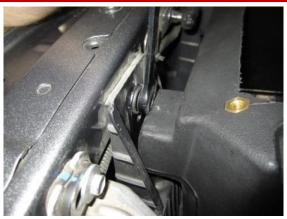
**6.** Locate one of the factory air box tray mounting bolts from removal step 7. Set CORSA air box into location and attach the bracket to the tray with factory bolt.
