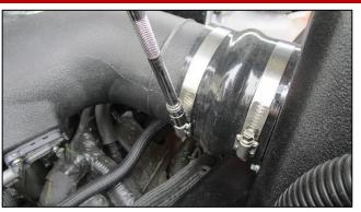
**8.** Adjust duct fitment as necessary and tighten all four clamps using a ratchet and 8mm socket.
