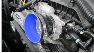
**6.** Place straight sleeve onto throttle body with included #64 clamp. Place included #64 clamp on other end of straight sleeve.
