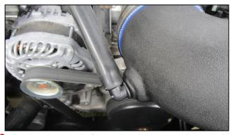
**10.** Push other end of breather hose onto installed elbow fitting in CORSA air duct.
