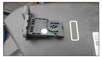
12. Remove factory gasket from MAF sensor.
