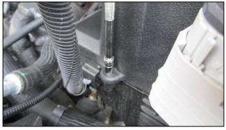
Install CORSA air box onto lower portion of factory air box in vehicle. Using the three factory screws from removal step 7, secure CORSA air box with a ratchet and 8mm socket with extension.
