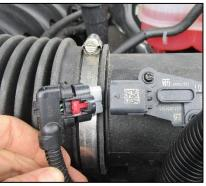
Pull red tab on MAF sensor wiring harness.
