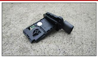
Install CORSA MAF gasket onto MAF sensor.
