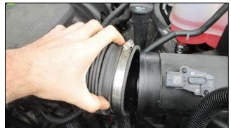
Pull air duct bellows from air box. Remove air duct from throttle body.
