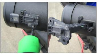
**11.** Remove two screws securing MAF sensor with a T20 Torx driver. Remove MAF sensor from factory air box.
