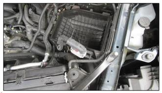
**10.** Lower factory air box remains in vehicle and is used with CORSA air intake.
