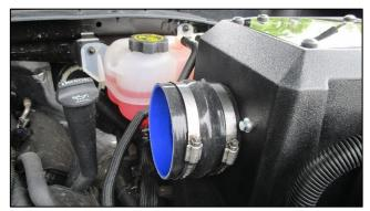
**5.** Place hump hose onto adapter with two of the included #64 clamps.
