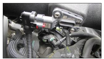
Re-route MAF wiring harness under large wiring harness and install into MAF sensor until it clicks into place. Push red tab back down to lock sensor in place.
