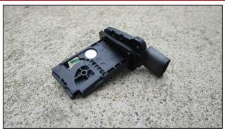
Install CORSA MAF gasket onto MAF sensor.
