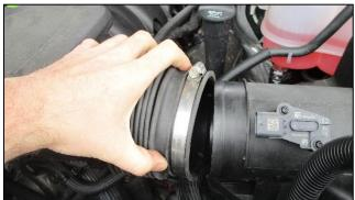
Pull air duct bellows from air box. Remove air duct from throttle body.
