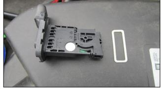
12. Remove factory gasket from MAF sensor.
