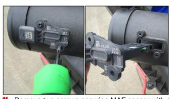
Remove two screws securing MAF sensor with a T20 Torx driver. Remove MAF sensor from factory air box.
