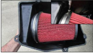
Install filter onto adapter in CORSA air box.
