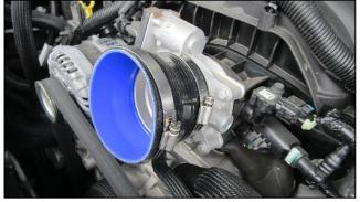
**6.** Place reducer onto throttle body with included #56 clamp on smaller diameter. Place included #64 clamp on larger diameter.
