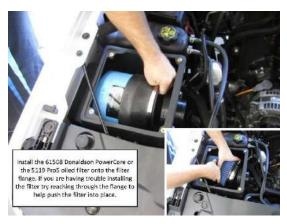
**3.** Install the air filter onto the filter flange. If you are having trouble installing the filter try reaching through the flange to help push the filter into place.
