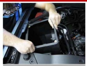
1. Place the CORSA box into the factory location.
