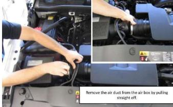
3. Remove the air duct from the air box by pulling straight off.
