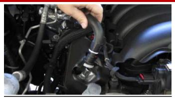
**6.** Remove the factory driver and passenger side breather hose from the engine.
