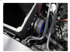
**5.** Attach the hump hose to the filter adapter using 5/16 socket or nut driver.
