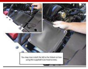
7. You may now install the lid to the CORSA air box using the supplied truss head screws.
