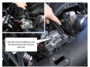
**10.** Press the shorter 5/8 hose onto the CORSA duct and crankcase vent line.
