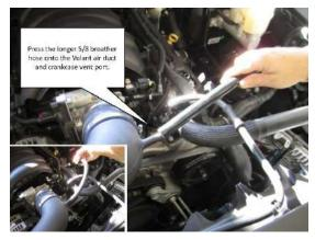
**9.** Press the longer 5/8 breather hose onto the CORSA air duct and crankcase vent port.
