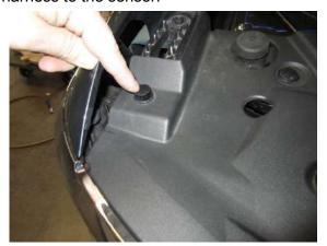
**16.** Reinstall the shroud support pins.
