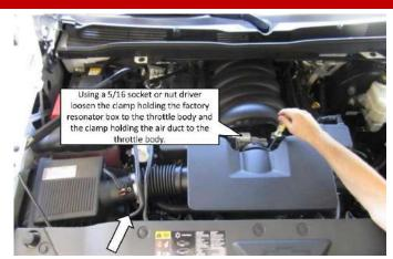
2. Using a 5/16 socket or nut driver loosen the clamp holding the factory resonator box to the throttle body and the clamp holding the air duct to the throttle body.
