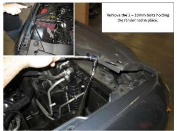
**11.** Remove the 2 – 10mm bolts holding the fender rod in place.
