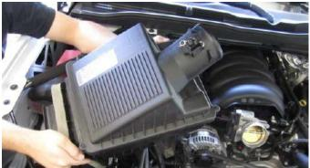
8. Remove the factory air box by pulling up and out.
