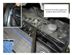
**15.** Reinstall the fender support rod using the factory 10mm bolts.
