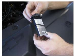
12. Remove the factory o-ring from the sensor. USE CAUTION! DO NOT TOUCH MAF SENSOR ELEMENTS. KEEP FREE OF DEBRIS.
