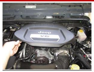
2. Remove engine cover by pulling up on the front then pulling cover out.
