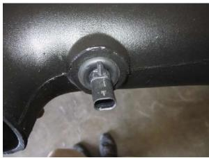
Locate the CORSA air duct. Push the air temperature sensor into the CORSA air duct.
