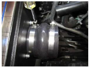
**6.** Locate the Ø3.5" hump hose and two #56 clamps. Install the hump hose along with one clamp onto the filter adapter and tighten clamp using a flathead screwdriver or ratchet and 10mm socket. Loosely place other clamp onto hump hose.
