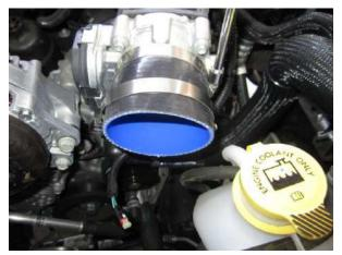
Locate silicone straight sleeve and remaining #56 clamps. Install straight sleeve along with one clamp onto throttle body and tighten clamp using a flathead screwdriver or ratchet and 10mm socket. Loosely place other clamp onto straight sleeve.
