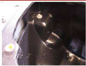
2. Locate bolt removed in removal step 10 and use it to secure air box into place. Tighten bolt using a ratchet and 10mm socket.
