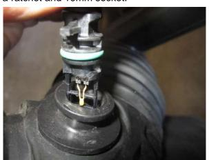
4. Locate the factory air duct and remove the air temperature sensor by gently lifting tab and twisting counterclockwise then pulling straight out.
