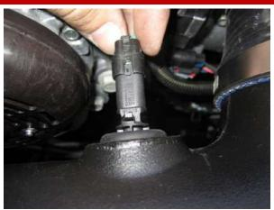
**11.** Reconnect the ATS wiring harness onto sensor. Push harness on until it clicks.
