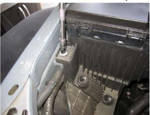
**10.** Remove the bolt in front of the fuse box using a ratchet and 10mm socket.
