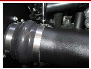
**9.** Tighten clamp on hump hose using a flathead screwdriver or ratchet and 10mm socket.
