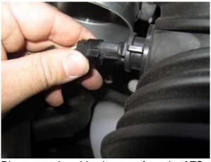
**6.** Disconnect the wiring harness from the ATS sensor on factory air duct.
