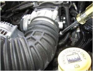
**5.** Loosen the clamp securing the air duct to the throttle body using a flathead screwdriver or ratchet and 8mm socket.
