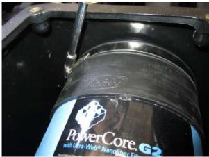
**3.** Locate CORSA air filter and install onto filter adapter inside air box. Tighten clamp using flathead screwdriver or ratchet and 8mm socket.
