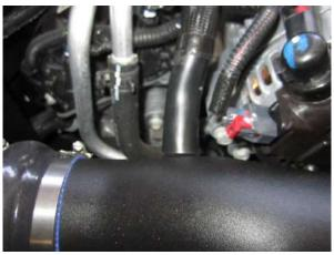
**10.** Install factory breather hose onto air duct.
