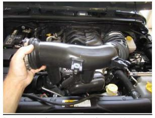
Remove the factory air duct from vehicle.
