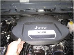
12. Locate the CORSA lid assembly and lid screws with rubber washers. Install lid onto air box and tighten screws with Philips screwdriver. Install engine cover. Check all hose connections and re-connect negative battery cable.
