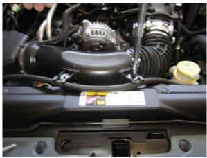
Remove the two bolts securing the factory air duct to the core support using a ratchet and 10mm socket.
