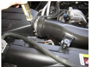
**4.** Loosen the clamp securing the factory air duct and box using a flathead screwdriver or ratchet and 8mm socket.
