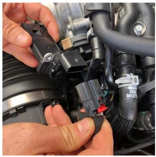
Unclip MAF sensor from wiring harness by pulling on the red tab. Set MAF sensor aside for installation
