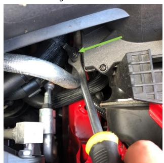
Use Trim Removal Tool to unclip the wiring harness retention clip located on the bottom left side of the airbox.
