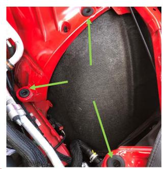
**8.** Remove factory air intake from engine bay. Make sure the 3 rubber grommets are not removed when pulling out the intake. Grommets are used during installation.
