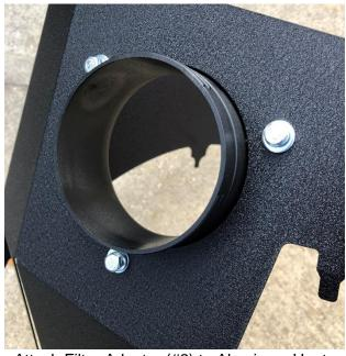
1. Attach Filter Adaptor (#2) to Aluminum Heat Shield (#14) as shown using the 3 washers (#11), lock washers (#12), and bolts (#10) using the 10mm socket and ratchet.
