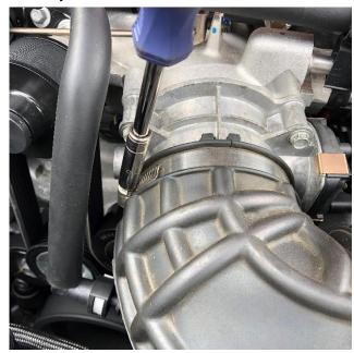
**4.** Loosen clamp to remove factory air duct from throttle body by using an 8mm socket.
