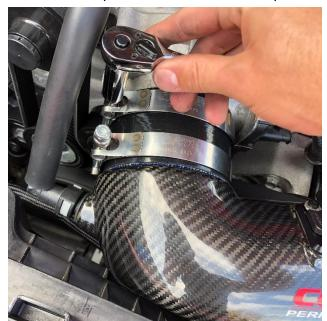
Tighten 4" T-Bolt Clamps to the air duct and throttle body using a 7/16" socket and rachet. NOTE: Take care to not over tighten clamps.
