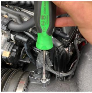
Remove MAF sensor screws using a T20 Torx bit or screwdriver.
