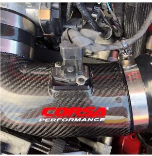
**10.** Reattach the MAF wiring harness to the MAF sensor. There will be a click when the harness is correctly inserted into the MAF sensor.
