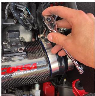
**8.** Tighten 4.375" T-Bolt Clamps on to the air duct and Filter Adaptor using the 7/16" socket. NOTE: Take care to not over tighten clamps.
