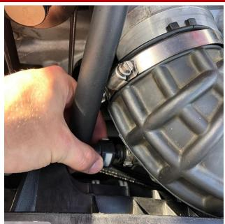
Remove breather hose from factory air duct by pressing on the light grey tabs on the quick disconnect fitting.
