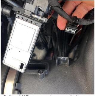
2. Pull out MAF sensor and remove clip from factory air duct.
