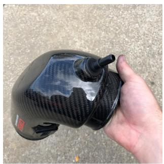
**3.** Install Rubber Grommet (#16) and Connector Fitting (#15) into the opening on the Carbon Fiber Air Duct (#1).
