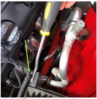
**6.** Unclip MAF sensor wiring harness from factory air box using the Trim Removal Tool.
