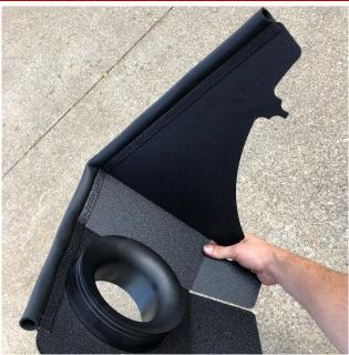
2. Attach Hood Seal Trim (#9) to top of Aluminum Heat Shield.
