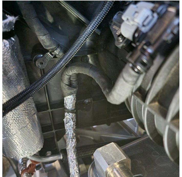
15. Pull the air box into the trunk as far as possible. Disconnect the wiring harness from the oblong shaped wiring harness retention clips, leaving the oblong portion of the clip attached to the air box.
