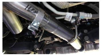
Next, rotate the Rear Adapter Pipe and slide the flared end of the Rear Adapter over the rear leg of the Single X-pipe. Do <u>not</u> slide the Sleeve Clamps on at this time. **INSTALLATION INSTRUCTIONS**
