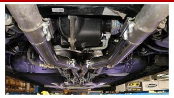
**16.** Once the entire exhaust system is properly adjusted, tighten all clamps to 45ft-lbs (61Nm) using the torque wrench and 15mm socket.
