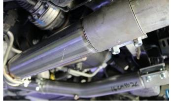
**13.** Note: If you are installing a CORSA Axle Back kit, complete its installation before continuing. When the CORSA Axle Back kit is installed, resume this installation. Slide the Sleeve Clamps over the compressed end of the Rear Adapters.
