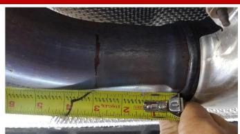
**6.** Starting on the Driver-side, measure  $2\frac{7}{8}$ , from the underside of where the Pipe welds to the factory secondary catalytic convertor, following along the underside profile of the Factory exhaust pipe. The tape measure must follow the bend profile of the pipe. Mark the pipe at the measured point to create a cut line.
