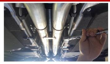
Snug the Clamp Nuts with a 15mm socket (or wrench), but do not tighten. Tightening now may hinder proper alignment of the entire system. These will be torqued later in the installation. Ensure the Clamp Nut and Stud are vertical while snugging
