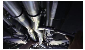
6. Locate the Single X-Pipe and 2 Clamps. Slide a Clamp over each front leg of the X-Pipe so that the nuts on the Clamps will located on the outside of the X-Pipe and face down, as shown in the next step. Slide the X-Pipe flared ends over the Drive and Passenger Head Pipe Adapters. The rear of the X-Pipe will need to be supported by a Jack Stand or similar until the Rear Adapters are installed.
