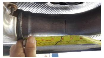
**1.** On the Passenger-side, measure  $4\frac{1}{8}$ " from the underside of where the Pipe welds to the factory secondary catalytic convertor, following along the underside profile of the Factory exhaust pipe. The tape measure must follow the bend profile of the pipe. Mark the pipe at the measured point to create a cut line.
