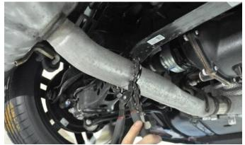
Using the Chain Style Pipe Cutter, cut both the Driver and Passenger Factory Exhaust pipes at the marked locations. The Factory Muffler will remain supported by the Muffler Grommets.
