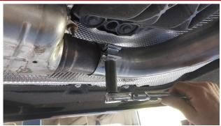
2. Snug the passenger side head pipe clamp to allow for minimal movement enough for adjustment.
