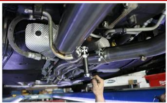
Snug the Clamp Nuts with a 15mm socket (or wrench), but do not tighten. Tightening now may hinder proper alignment of the entire system. These will be torqued later. Ensure the Clamp Nut and Stud are vertical while snugging.
