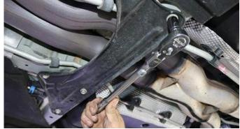
Then reinstall the Cross Member with a 13mm socket (or wrench) and the 5 Factory bolts. Tighten all bolts to the manufacturer's specifications.
