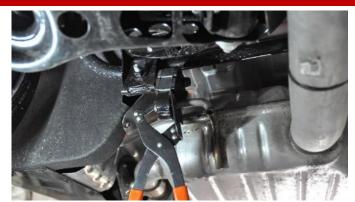
5. Note: If you are installing a CORSA Axle Back kit, skip this step and refer to Steps 3 and 4 in the Removal section of the CORSA Axle Back instructions. Remove the two Hangers on the rear each side from the Factory Grommets using the Exhaust Hanger Removal Pliers or a similar device. <u>Note:</u> Careful not to damage the Grommets during removal. (Will be reused during installation)
