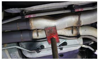
**4.** Support the Factory Crossover Pipe using a jack stand or similar device.
