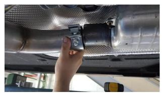
**3.** Locate new Driver-side Head Pipe and slide it into the factory cut pipe with the clamp as shown.
