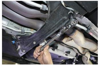
Remove the 5 bolts connecting the Cross Member with a 13mm socket (or wrench). Store the Bolts and Cross Member in a safe location. They will be reinstalled during installation.
