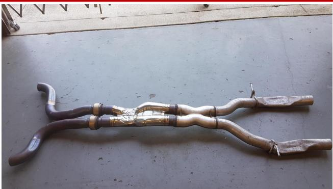
**10.** With assistance, put the cut section of the factory exhaust away
