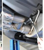
**1. CAREFULLY** insert the tip assembly into the driver side muffler outlet pipe and snug the clamp using a 15mm socket, 3/8" driver ratchet and 3" extension.
