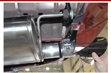
CAREFULLY remove the tip assembly from the mufflers to free it from the vehicle.
