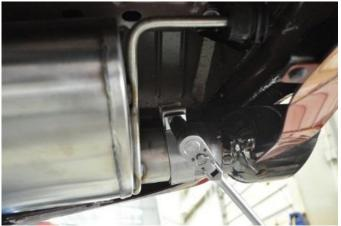
Loosen the two clamp bolts at the inlet of the current CORSA driver and passenger tip assemblies using a 15mm socket and a 3/8" ratchet, and a short extension.
