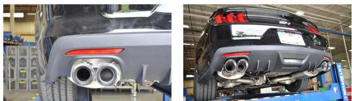
**3.** Adjust the position and depth of the tip assemblies until it is centered in the cutout, and has an equal amount of reveal on each side, then tighten the clamps using a 15mm socket and 3/8" ratchet. Torque the clamps to 45ft-lb using a torque wrench and 15mm socket, ensuring that the tips are still in the desired position.
