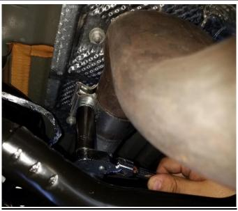
Loosen the factory clamp at the inlet end of the factory rear muffler assembly using a 15mm socket.
