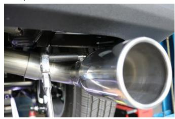
**9.** Visually inspect the exhaust system position, tip alignment, clamp orientation, and exhaust pipe clearance. Make any necessary adjustments at the slip joints.
