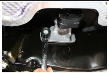
Re-install the driver and passenger hanger assemblies back in to their respective positions.
