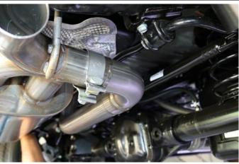
**4.** Slide the expanded inlet end of the rear muffler assembly onto the front section. Note: Make sure the clamp is on before you do this.
