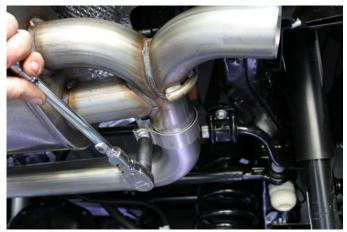
**5.** Using a 15mm socket or wrench, snug the clamp before the muffler assembly, but do not tighten completely.
