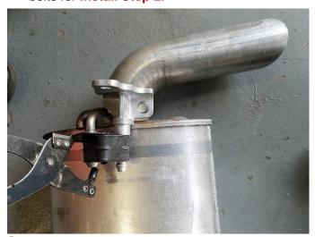
4. Using a grommet puller or similar device, remove both hanger grommets from the factory rear muffler assembly. Note the position and orientation of each hanger assembly before removal and save for Install Step 2. NOTE: The use of a soap and water solution may aid in removal of grommets.
