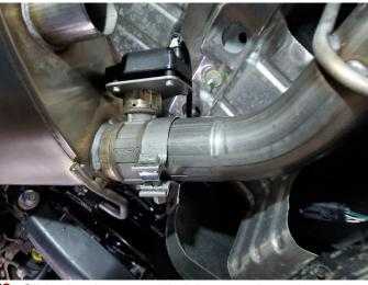
**16.** Slide the tip assembly inlet onto the valve outlet of the muffler.
