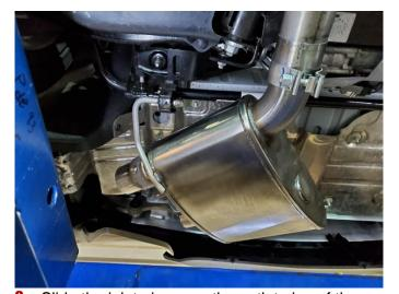
Slide the inlet pipe over the outlet pipe of the stock exhaust.
