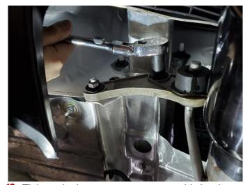
18. Tighten the hanger grommet assembly hardware using a 15mm socket and 3/8" ratchet. Repeat steps 12-18 for the driver side outer tip assembly.
