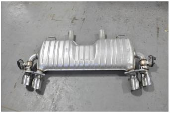
Push up slightly on the exhaust, and then slide the stock rear muffler rearward to free the rear grommet assemblies from their mounting on the chassis. This will free the rear muffler from the vehicle.
