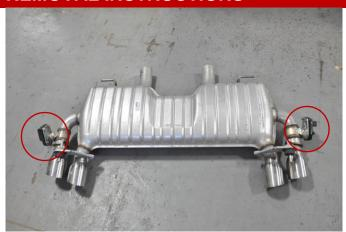
**9.** Remove the three screws securing each valve control unit to the outer stock tips using an 8mm socket and ¼" ratchet. Label each unit with the position it was installed to make sure it goes back to the same location.
