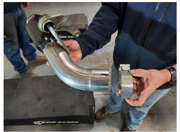
14. Locate one of the 3" clamps and slide the clamp onto the inlet of the tip assembly. Orient the clamp so the bolt is vertical with the nut towards the ground and the bolt towards the inside of the vehicle.
