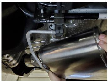
Slide the muffler hanger into the hanger grommet 6.
