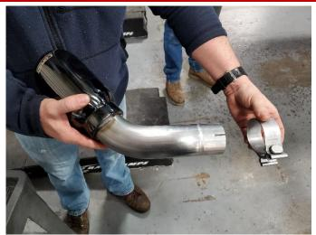
**19.** Locate the passenger inner tip assembly and one 2.25" clamp and slide the clamp onto the inlet of the tip assembly. Orient the clamp so the bolt is vertical with the nut towards the ground and the bolt towards the inside of the vehicle.
