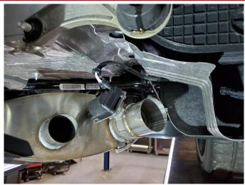
Connect the other end of the extension to the valve control unit. Press down gray locking tab to secure. Repeat steps 4-11 for the driver side muffler.
