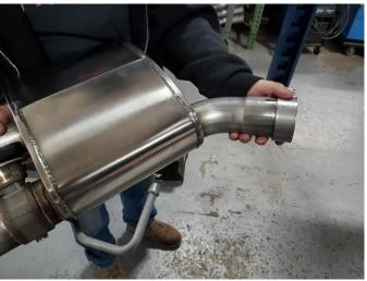
4. Locate one of the 2.75" clamps and slide over inlet of the passenger muffler. Orient the clamp so the bolt is vertical with the nut towards the ground and the bolt towards the inside of the vehicle.
