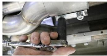
3. Install the outlet of the CORSA X-Pipe assembly into the factory sleeve clamps at the inlet of the axle pipes. Using a 15MM socket or wrench to snug the 2 bolts on the sleeve clamp. Repeat for opposite side
