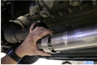
5. Adding a 2.75" clamp to the inlet side of each CORSA Inlet Elbow Pipe.
