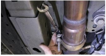
Using a 13MM socket or wrench, loosen the spherical clamps at the inlet of the H-pipe on the passenger side and driver side.
