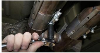
Using a 15MM socket or wrench, loosen the factory sleeve clamps (4 Bolts) after the H-Pipe assembly.
