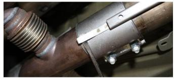
**3.** On the driver side, use a flat screwdriver to pry the clamp spring clip from the retainer pin on the H-Pipe repeat on passenger side.
