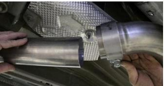
4. Add a 2.75" clamp to each of the CORSA X-Pipe inlets. Insert the CORSA Inlet Elbow Pipes into the X-Pipe inlets. Snug connection using a 15mm socket or wrench.
