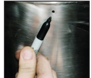
Fig 1. NOTE: IMPORTANT: Make sure that small drain holes of each tunnel muffler face down when installed.
