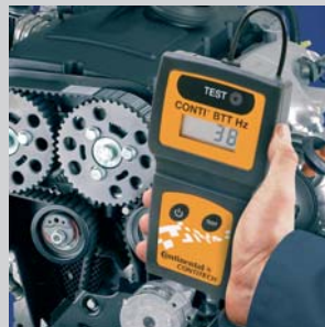
CONTI® BTT Hz (Belt Tension Tester): Electronic alternative for measuring the tension of multiple V-ribbed belts
