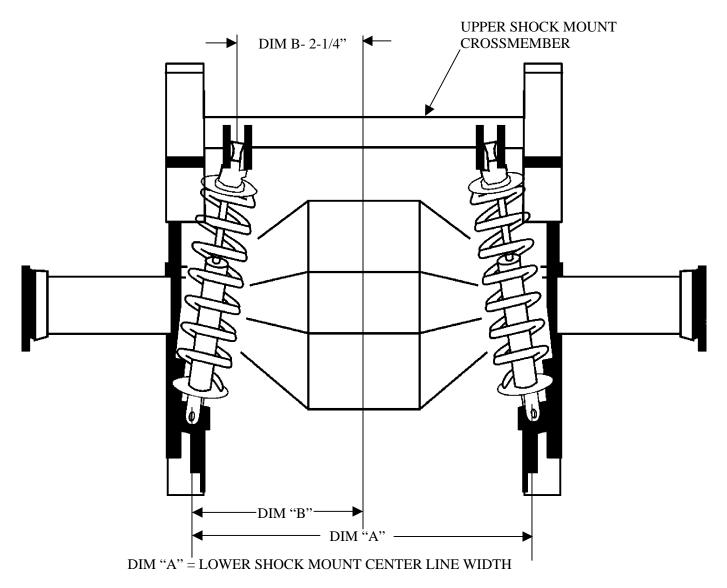
DIM "B" =  $\underline{\text{DIM "A"}}$
