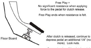
Over extension of the clutch pedal will cause damage.
