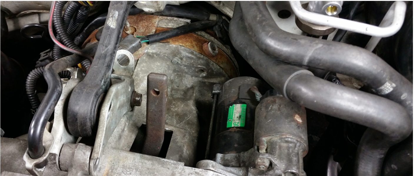
Factory release hydraulics removed closeup
