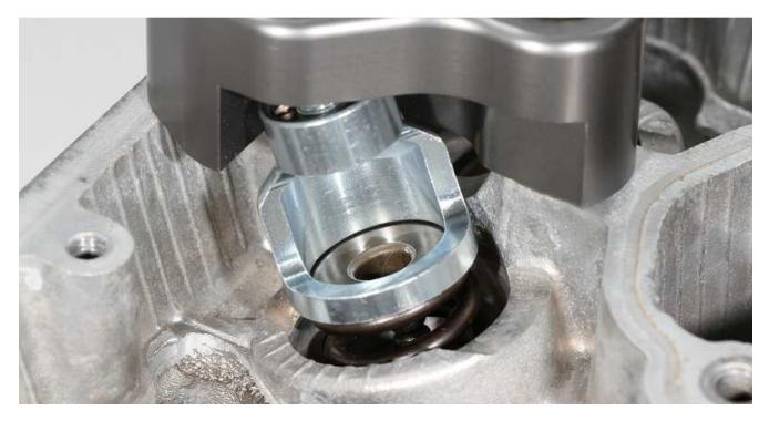
Step 7) You can now remove the spring and retainer. This will allow the valve and/or the valve stem seal to be removed and installed.
