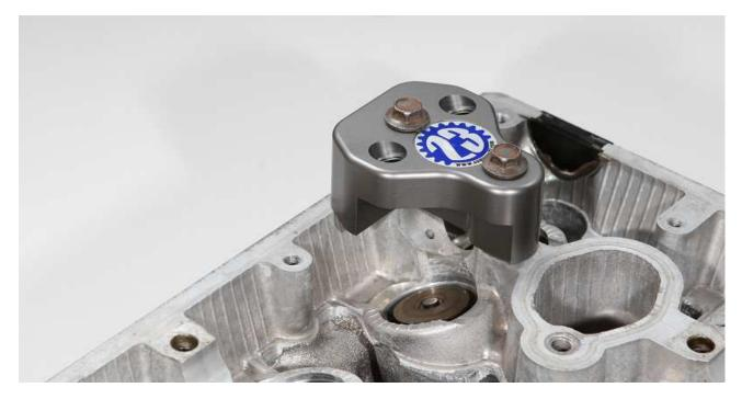
Step 3) Thread the tool stud into the threaded hole with the internal 5mm hex on top. Install the spring cage under the stud as show n.
