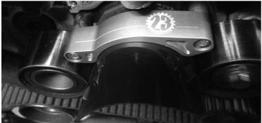
Step 5) Remove the Company23 Timing Belt Guide Spacer Tool.
