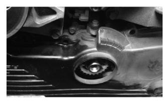
Step 2) Remove the timing belt guides. On manual transmission cars, you will need to remove the factory belt guide using a 10mm socket. If you are changing the timing belt at the same time, follow those steps now. (See Company23 Cam Lock Tool #506 Manual for more)
