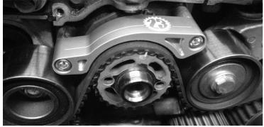
Step 4) Insert the supplied Company23 Timing Belt Guide Spacer Tool between the timing belt and guide. Press down on the belt guide so that there is an even gap around the belt that is the thickness of the spacer tool. Tighten the bolts to 9.8Nm (1.0kgf-m, 7.2 ft-lb) using a 5mm socket. WARNING: DO NOT OVERTIGHTEN THESE BOLTS!
