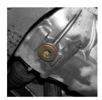
**2.** For 07 WRX STI with a 6sp manual transmission that utilize a torx T70 transmission drain plug: Remove and install drain plug using the Company23 Torx T70 socket. Bolt torque is 44 Nm (4.5kgf-m, 32.5 ft-lb)
