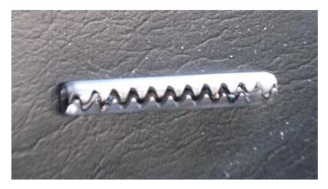
Step 3) Tap the Company23 roll pin tool to install the new axle pin. The pin should be installed flush with the CV axle's outside diameter. Twist the tool as you remove it.
