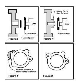
area shown in figure 1 will rub against the back side of the camshaft timing gear. The camshaft retaining plate should not come into contact with any part of the camshaft gear sprocket area. The only contact area between the camshaft retaining plate and the timing gear should be in the hub area.
