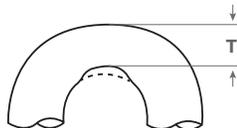
Measure cross section at link ends to determine wear. If chain is worn to less than the minimum allowable thickness, remove from service.
