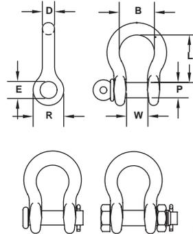
**STYLES:** Screw Pin, Round Pin, Bolt/Nut/Cotter
