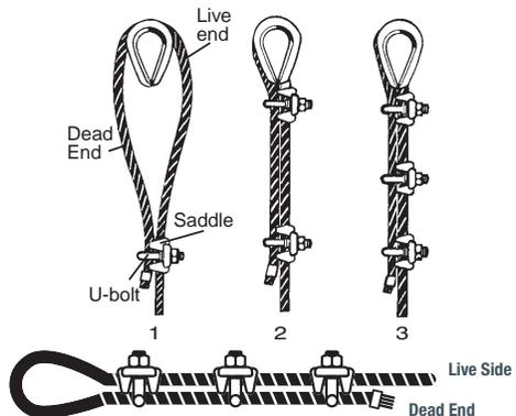
NOTE: Mechanical spliced or finished eyes slings are the preferred method of wire rope sling construction. OSHA does not allow the use of clips to form the eyes of wire rope slings.
