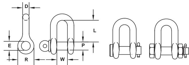
**STYLES:** Screw Pin, Round Pin, Bolt/Nut/Cotter
