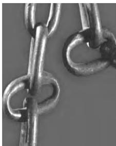
Figure 3 : Inspection for interlink wear can be detected easily by collapsing the chain.
