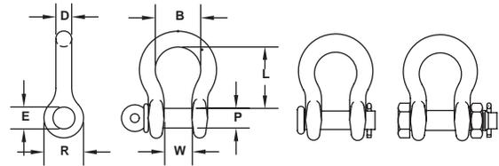
**STYLES:** Screw Pin, Round Pin, Bolt/Nut/Cotter
