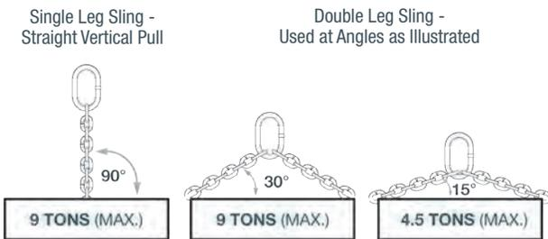
Working load limits for 5/8 inch alloy steel chain slings, (single and double leg configurations.)
