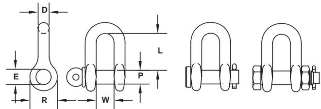
**STYLES:** Screw Pin, Round Pin, Bolt/Nut/Cotter
