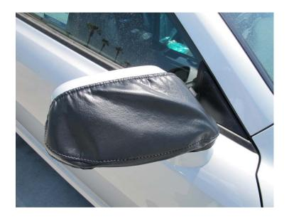
4. Pinch the neck of the mirror with left hand and pull Velcro loop down with right hand towards Velcro hook at the bottom of the mirror cover and attach Velcro to hold it in place
