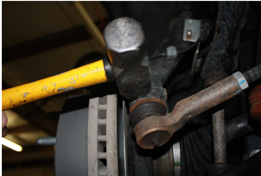
Figure 9: remove passenger tie rod from spindle
