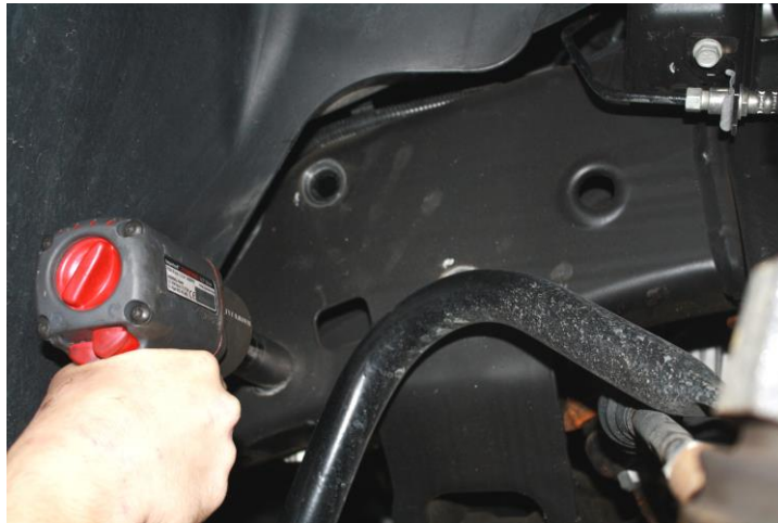
Figure 6: unbolt steering box from frame
