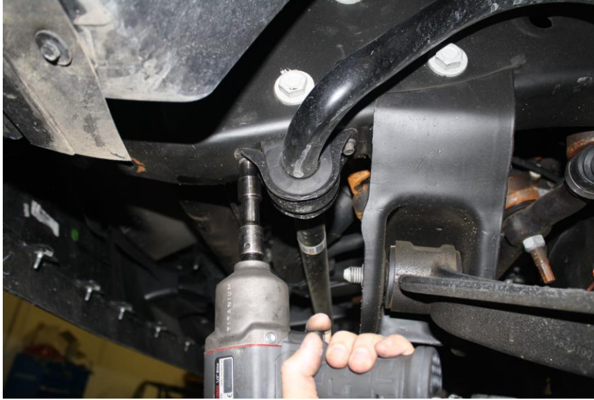
Figure 3: unbolt sway bar from frame
