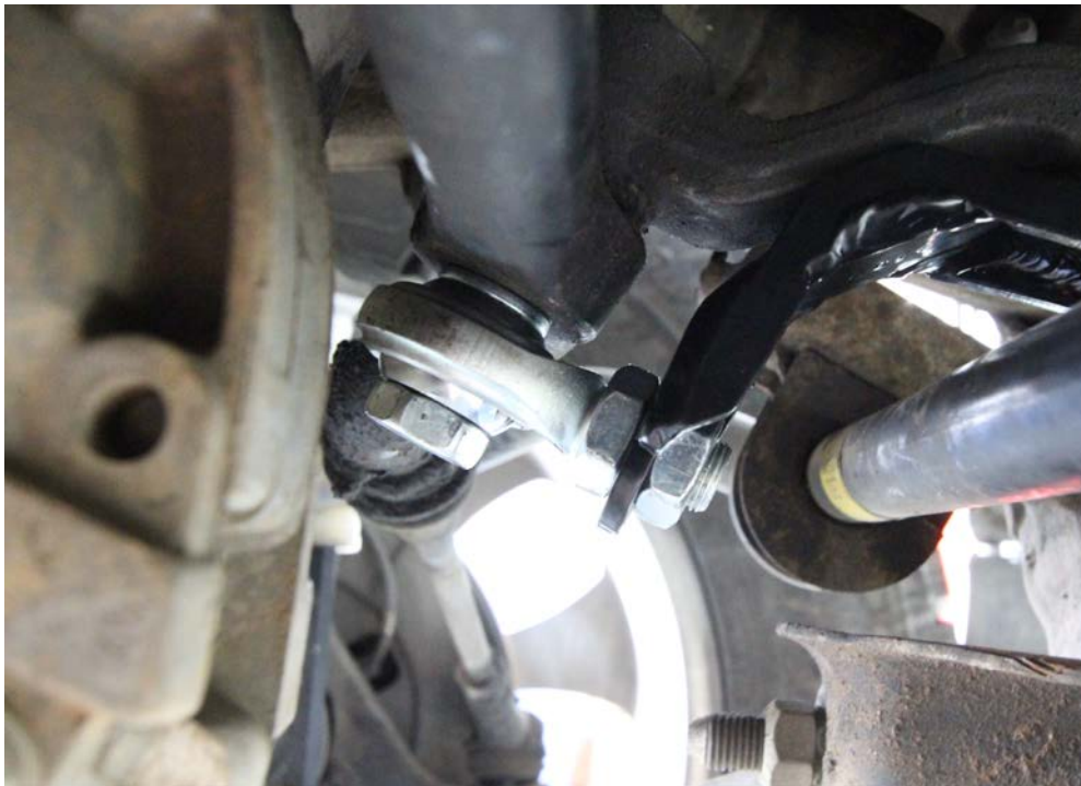
Figure 6: pitman arm bracket installed
