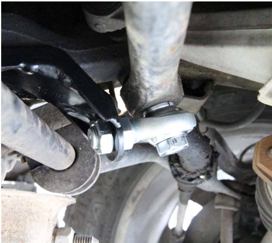
Figure 4: idler arm bracket installed
