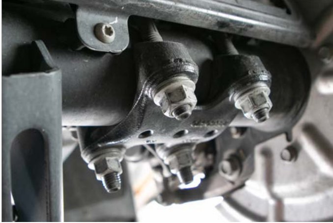
Figure 2: Remove Factory U-bolts
