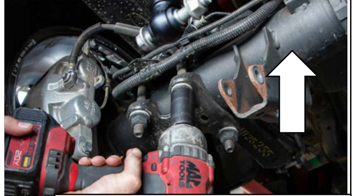
Figure 2: Remove Factory U-bolts
