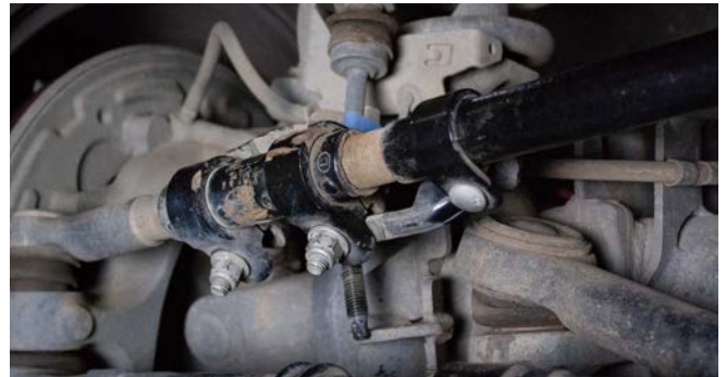
Figure 12B: Steering Link Adjuster Secure
