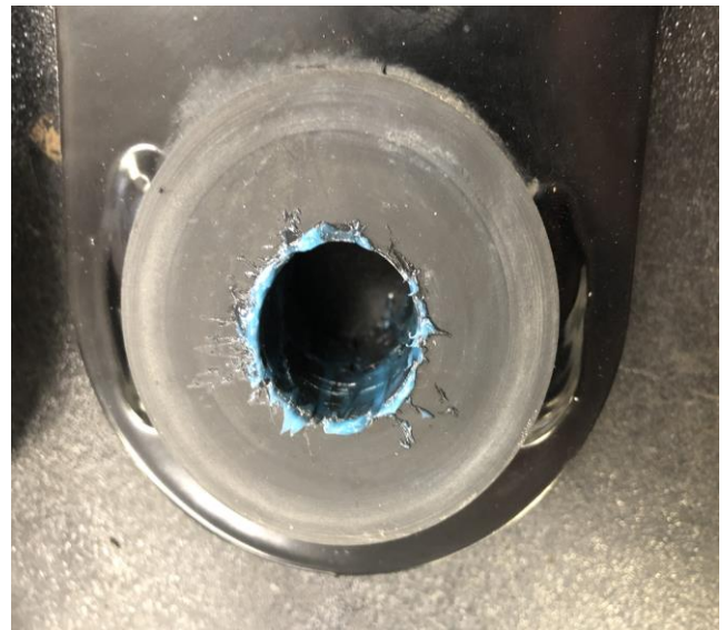
Figure 13: Grease Shackle Bushings
