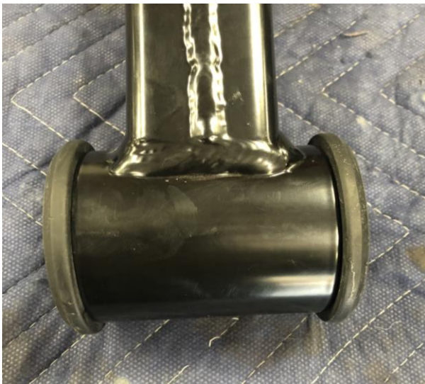
Figure 21: Traction Bar Bushings Installed
