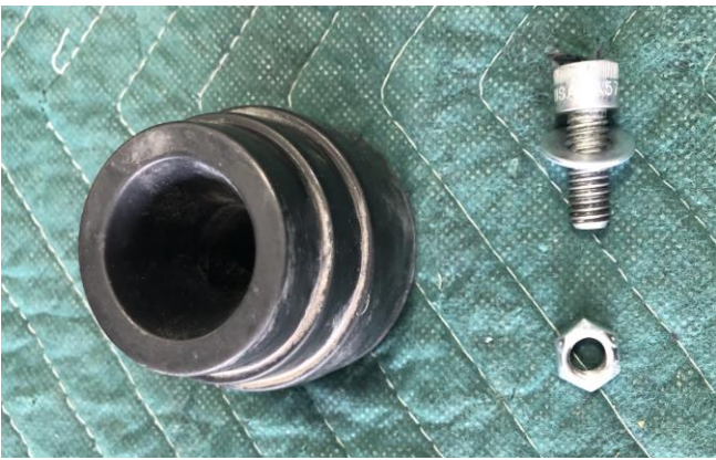
Figure 7: Bump Stop Mounting
