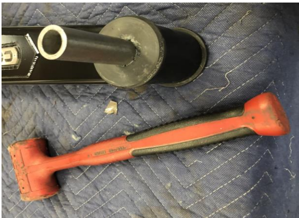
Figure 4: Install Radius Arm Crush Sleeves
