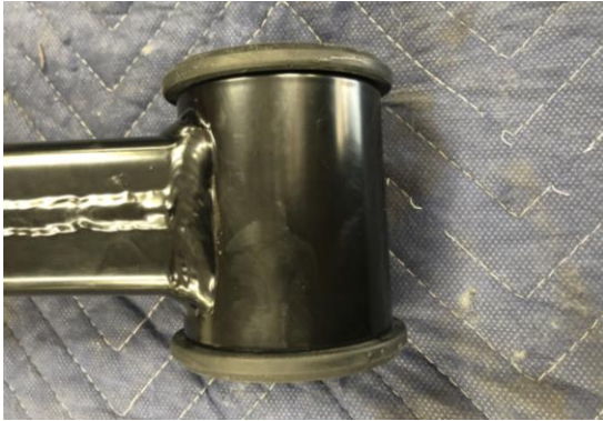
Figure 2: Install Radius Arm Bushings
