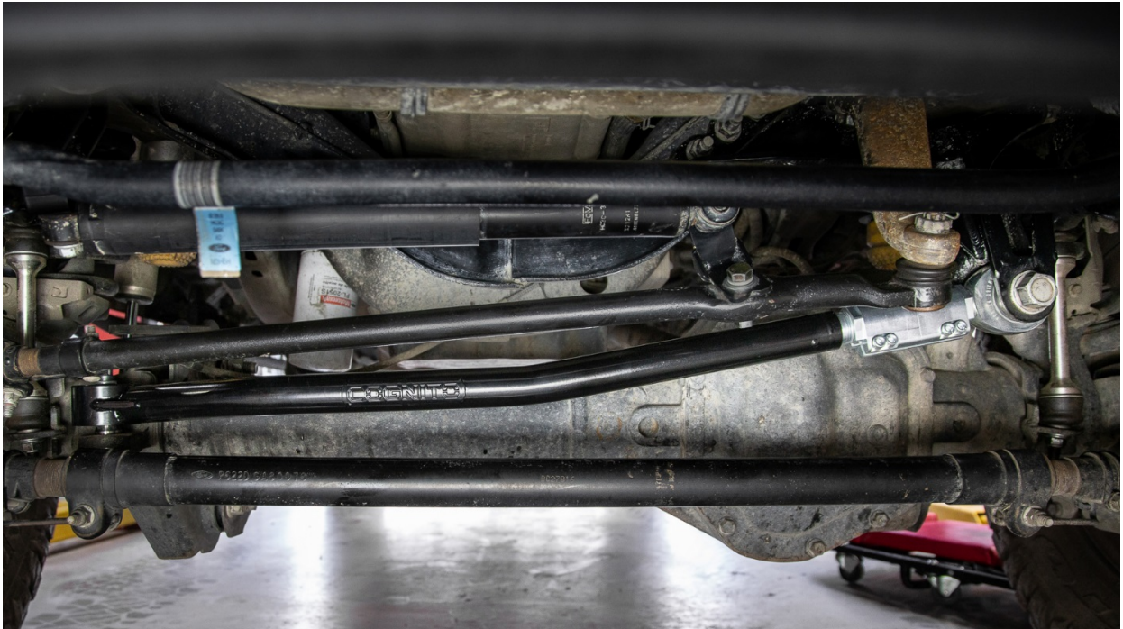
Figure 22: Installed Track Bar
