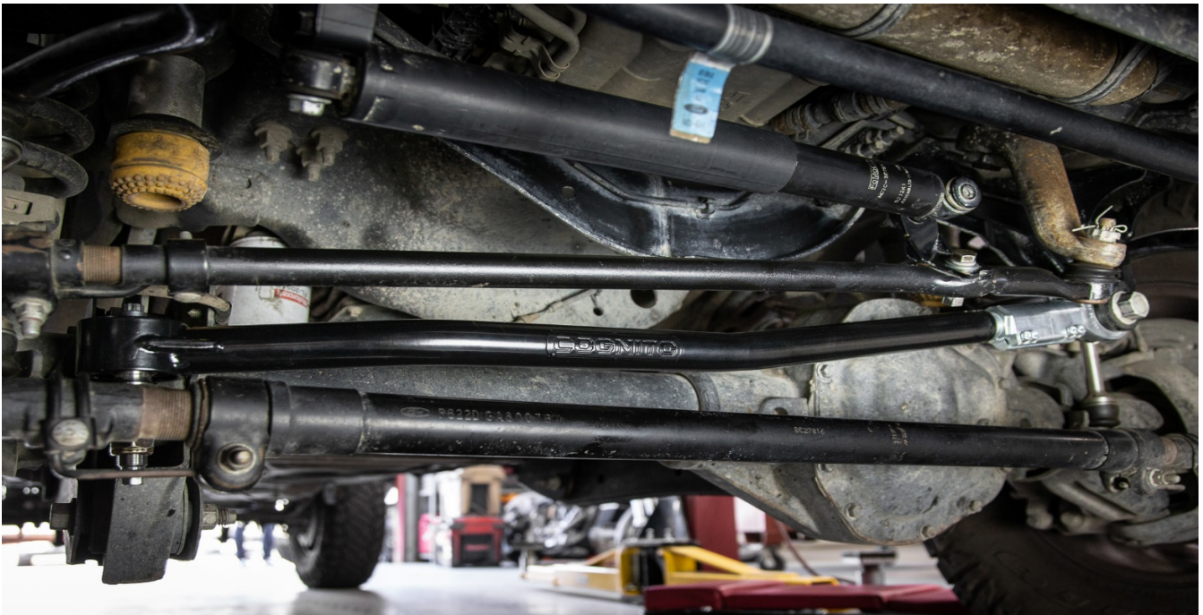
Figure 21: Installed Track Bar
