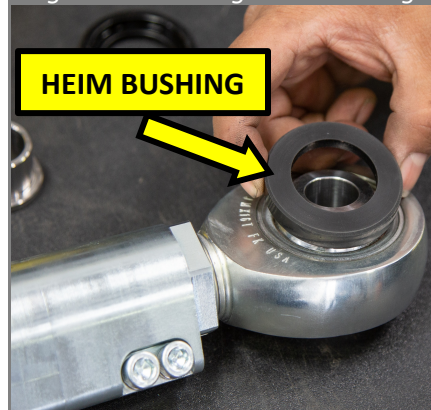
Figure 8: Installing Heim Bushing
